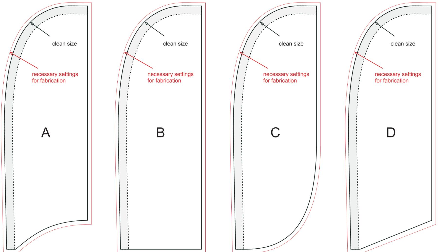
The grey arc in the template shows the underlay and stitching of the rod tunnel - we do not recommend placing smaller graphics, texts or logos in this space, as they could be slightly deformed by stitching.
